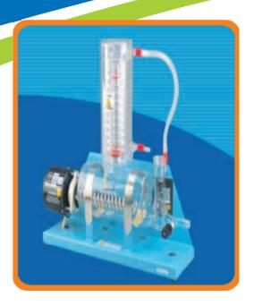
Ideal for general laboratory use capable of providing pyrogen free water
